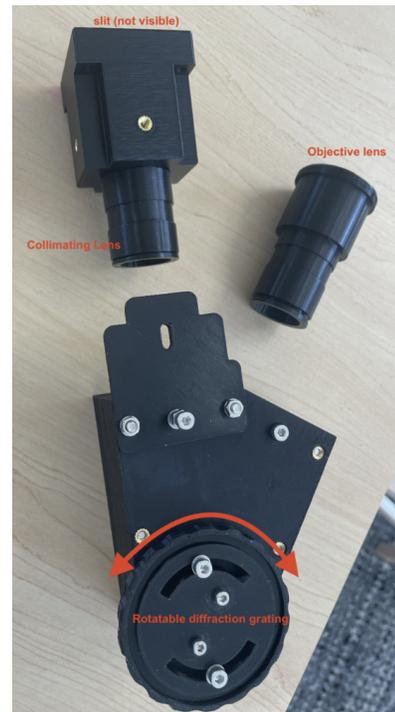
FIG. 10. 3D-printed spectrograph model showing individual components and their spatial configuration made by *Sol'Ex* [2], respectively
