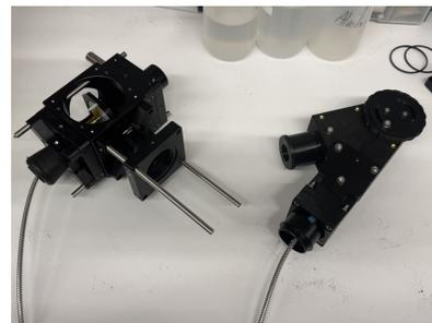
FIG. 11. Left: Finalized prototype with the appropriate components. Right: the 3D-printed spectrograph connected with the fiber optic cable
