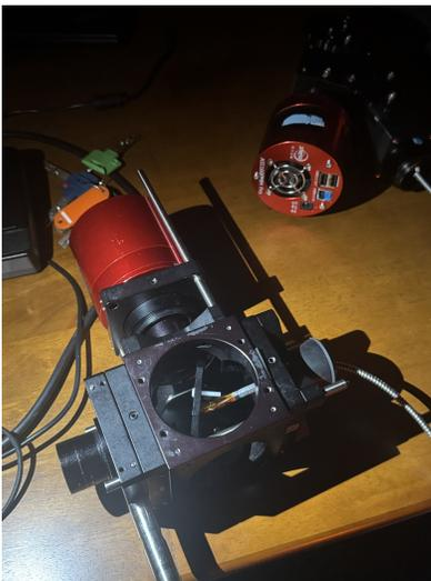
FIG. 9. Thorlabs beam-splitter cube with the cage plates, guider camera, and fiber optic cable
